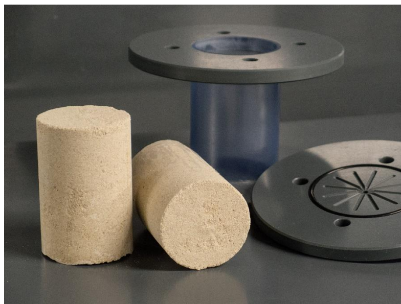
Figure 3: The solid columns that were produced using MICP and synthetic, stabilized urine.
